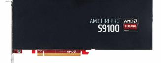
Compute-intensive workloads are no challenge for AMD FirePro<sup>®</sup> S9100 server GPUs. With support for OpenCL<sup>®</sup>, 12GB GDDR5 memory and ECC memory support, up to 2.11 TFLOPS of peak double-precision floatingpoint performance and up to 9.4 GFLOPS per-watt peak double precision performance, it's clear the AMD FirePro S9100 is a high-performance computing powerhouse.
